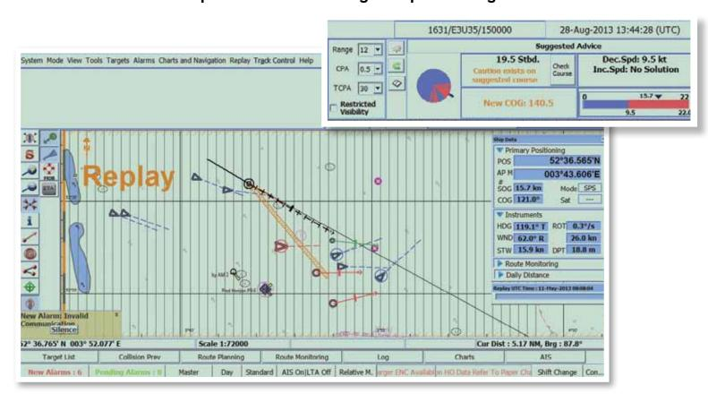
The advice given is in full compliance with International Regulations for Preventing Collisions at Sea 1972 (Colregs). The innovative technology has been designed to assist the OOW in making correct decisions based on all available data from AIS and ARPA.
